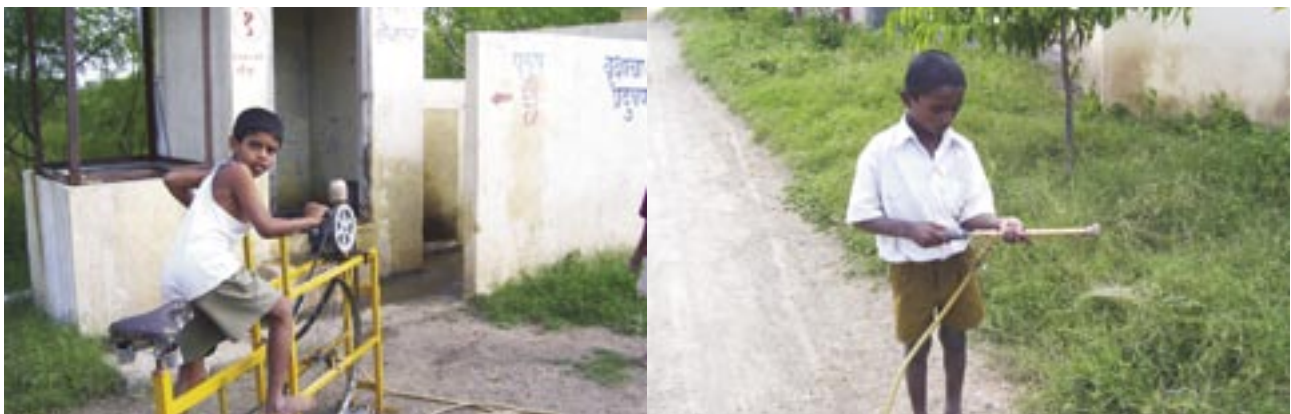
Greywater pumping by cycle pump and its use for gardening
